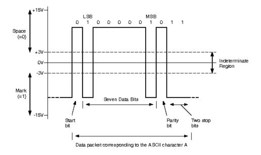
**Serial** Interface only needs one I/O to communicate. However, Parallel Interface takes eight or even more. For example, Analog / digital converter and digital / analog converters, LCD and temperature sensors all supported to Serial Interface.
